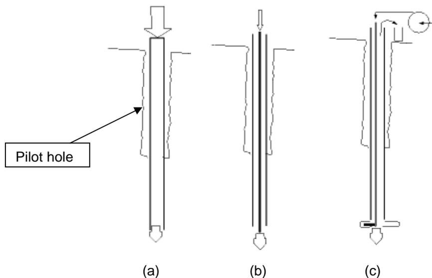
Figure 6a-c. Expose the borehole (a); notch the borehole (b) and nucleate the fracture by applying pressure to the well (c) (From [www.frx-inc.com](http://www.frx-inc.com)). The sump is not shown in this sketch. Remark: In the STRESOIL project has the fracturing wells been installed without pilot holes to minimize the risk for by pass flow of injected steam along the outer side of the casing.
