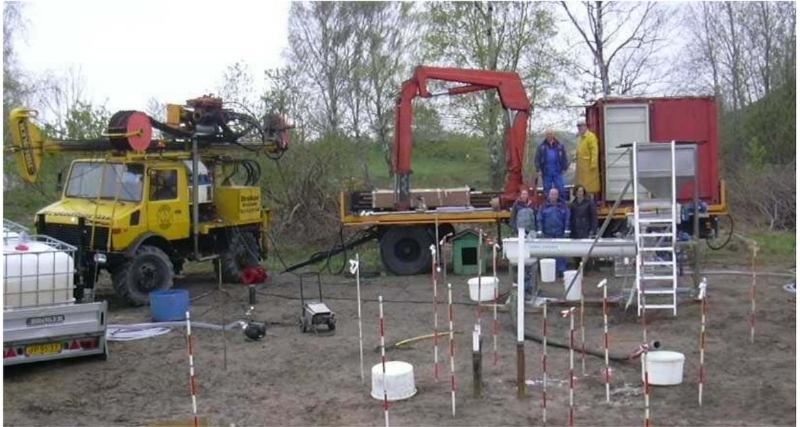
Figure 5. Survey measurements of terrain uplift during injection of hydraulic fractures in the subsurface
