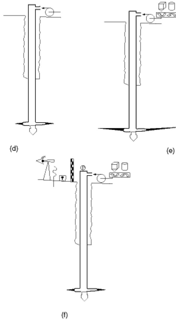
Figure 6 d-f. (d) Initial fracture propagation; (e) further development of fracture and (f) monitoring of slurry pressure / rate and surface uplift (From [www.frx-inc.com](http://www.frx-inc.com)).
