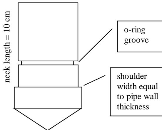
Figure 1a. Schematic of Drive Point
