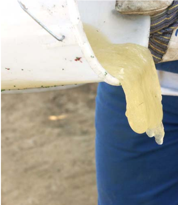
a) Guar gel, borax and breaker solution
