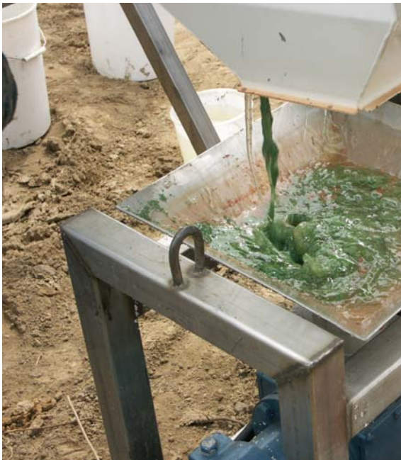
c) The slurry discharged from the mixer into the small receiving hopper
