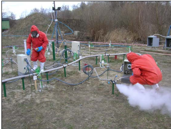
Figure 4: Testing of the steam remediation set-up
