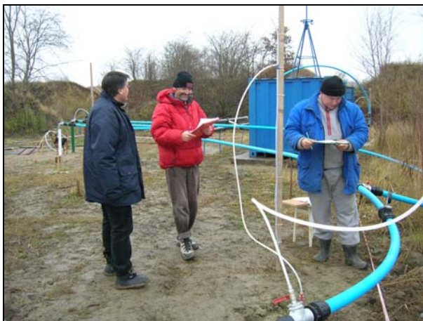
Figure 3a: Air pressure permeability test
