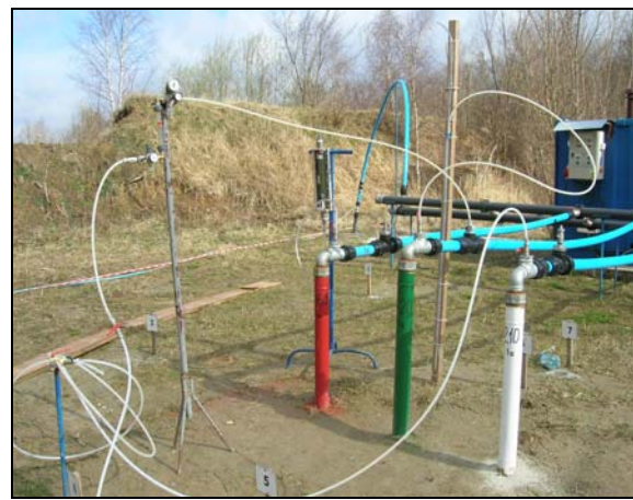
Figure 3b: Air pressure-flow test
