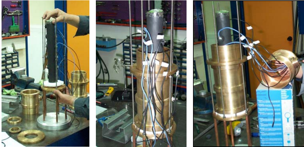
Figure 5: Photographs showing details of the connection of electrodes inserted in undisturbed soil samples with external conductivity meter.
